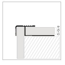
Scala-T has matte anodized, bright anodized, satin chemical bright anodized and electrostatic powder painting options. While silver, yellow, inox, bronze and black anodized color coatings are available, it can also be painted to the desired RAL code with electrostatic powder painting.
