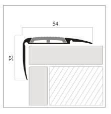
Scala-R has matte anodized, bright anodized, satin chemical bright anodized and electrostatic powder painting options. While silver, yellow, inox, bronze and black anodized color coatings are available, it can also be painted to the desired RAL code with electrostatic powder painting.
