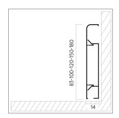
Lato has matte anodized, bright anodized, satin chemical bright anodized and electrostatic powder painting options. While silver, yellow, inox, bronze and black anodized color coatings are available, it can also be painted to the desired RAL code with electrostatic powder painting.
