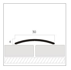
Curvo has matte anodized, bright anodized, satin chemical bright anodized and electrostatic powder painting options. While silver, yellow, inox, bronze and black anodized color coatings are available, it can also be painted to the desired RAL code with electrostatic powder painting.
